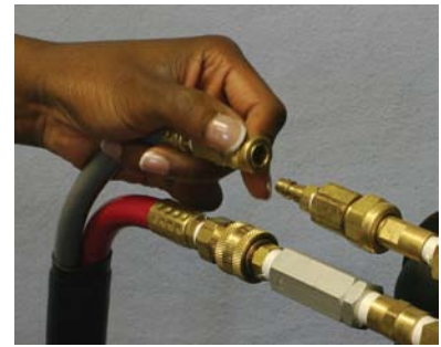
To connect or disconnect the air or liquid connections on the spray gun, pull back the outer sleeve of the socket to release.
