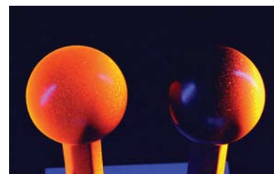
A picture worth a thousand words... In this test, fluorescent dye has been sprayed on two round knobs. The left knob was sprayed with the electrostatic system ON; the right knob was sprayed with the same sprayer, but with the electrostatic system OFF. Note how even the coverage is on the electrostatic knob.
